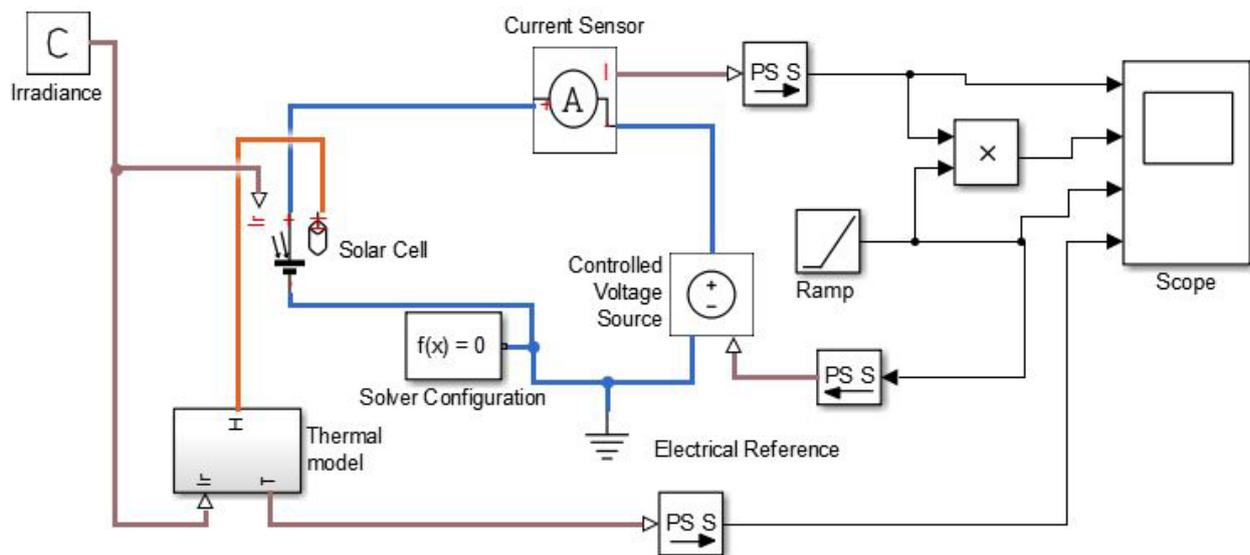
**Fig. 4** - Simscape-model for researching the solar cell
